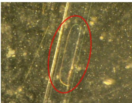
Figure 4.2 Bubble in sample channel.
